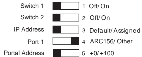
Figure 16. BACLink DIP Switches
