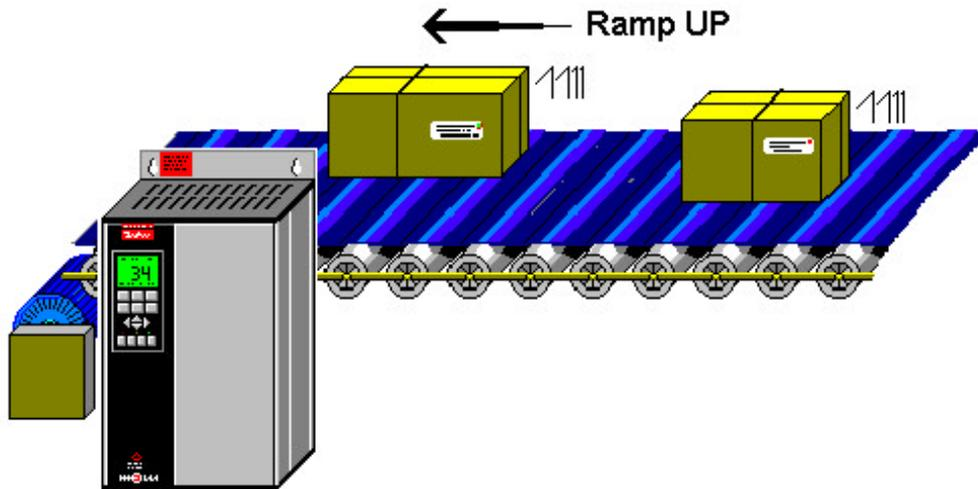
A ramp is also present on the stop side. This is referred to as a ramp down or deceleration. It is important that packages are not jerked to a halt. A ramp-down of 10 seconds might be entered into the program for this application. If the ramp is too short, the drive can trip on over voltage.
