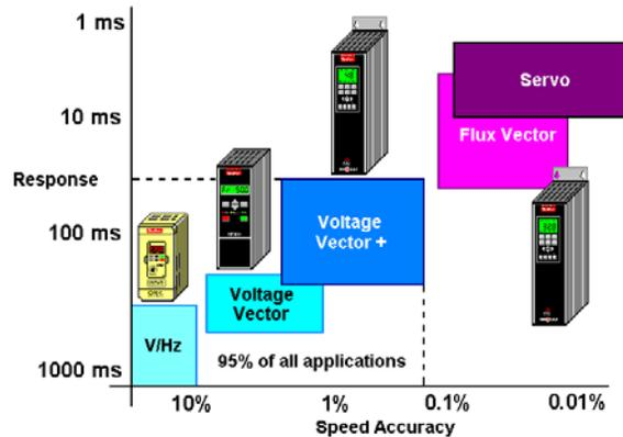
There are different types of AFDs, which are briefly covered here. They include Volts/Hz, Voltage Vector, Voltage Vector +, Flux Vector and Servo.
