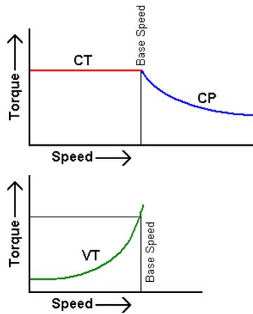
This part of the lesson covers the application terminology associated with an AFD, starting with application torque curves.
