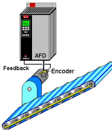
Speed Closed Loop requires an encoder to feedback the RPM signal to the AFD letting it know the speed of the motor.
