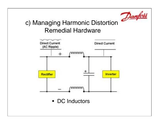
Another way to reduce harmonic noise is to use DC inductors or chokes built in the drive. These eliminate some of the noise, usually about 40%. This method is what Danfoss uses, building DC inductors into all of its drives. These DC inductors are expense which has caused most VFD manufacturers to offer them as options.
