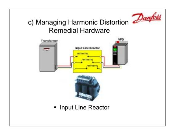
One of the most common remedies used by many drive manufacturers is to place an input line reactor (between 3% to 5%) between the drive and the power supply. This does reduce the harmonic noise, but it also reduces the voltage going to the drive. This reduced voltage might be a problem when the drive is used at maximum load and maximum speed. The motor can become voltage starved. This might require the VFD to be a size larger to avoid nuisance tripping.
