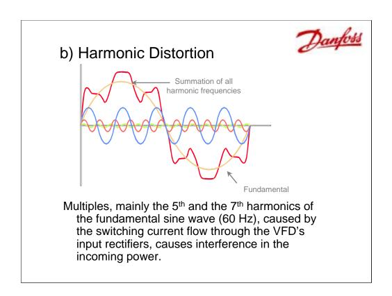
Harmonic distortion has been a hot topic in North America with the ever increasing use of equipment incorporating rectifiers and similar switching devices on the input. This noise is low frequencies that appear on wires coming from the supply transformer.
