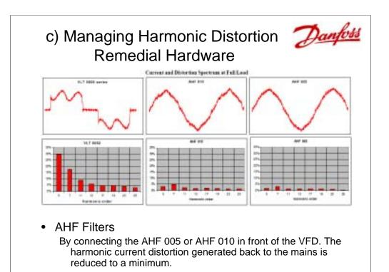
In the diagrams above the bar chart to the left shows the amounts of current distortion on a 6-pulse drive that has DC inductors. When the AHF filters are placed upstream from the VFD, notice in the middle chart and the chart on the right that the harmonic levels are very small. Another advantage that the filters have over a 12-pulse VFD is there is only a slight increase in harmonics on the power when there is a phase imbalance.
