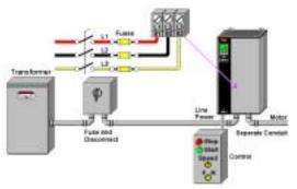
This lesson covers the terminology associated with the incoming power to a Variable Frequency Drive (VFD) and the efforts to protect both the VFD and incoming power.
