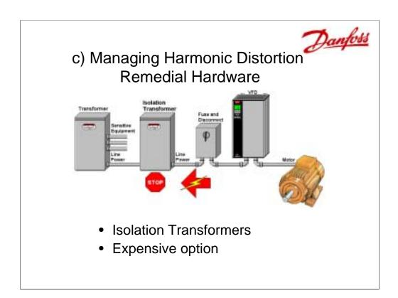
Another option to stop harmonic noise is to place an isolation transformer between the drive and sensitive equipment. Most of the noise if engineered correctly stops at the isolation transformer. This can be a very expensive option. In the past, many drive manufacturers required isolation transformers to prevent ground faults and protect against uneven phase to ground voltages.
