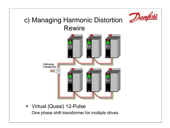
One way to avoid the more expensive 12-pulse drives is to wire the drives in a virtual or quasi 12-pulse configuration. Here a large 30° phase shift transformer is used to power 2 sets of VFDs, one from the standard part of the transformer and the other from the 30° phase shift part. This allows the use of the much less expensive 6-pulse drives with the harmonic cancellation advantages of the 12-pulse.
