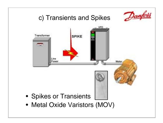
Another problem that might be encountered with incoming power is spikes or transients of voltage, which occur for a very short amount of time. These spikes may be caused by heavy loads in the main supply being switched ON then OFF, or even by lightning strikes. A VFD must have the capacity to handle these spikes in the same way that personal computers need surge protection.
