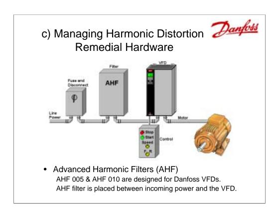
Another option is to use a harmonic filter as pictured above. This device is mounted between the drive and incoming power and it reduces harmonic noise problems. These filters can be passive or active. The one pictured above is a passive filter specifically designed to work with Danfoss drives and their DC inductors.
