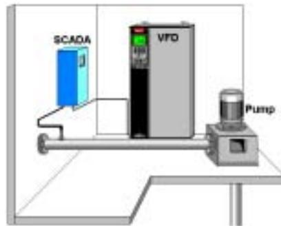
**VFD controls water flow.**
