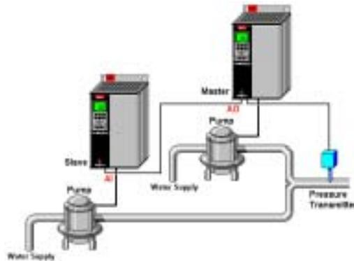
In the Master/Slave arrangement a Master or Lead VFD monitors the pressure sensor and operates a single pump. It sends a corresponding signal to another following pump. Features of the VFD which were restricted in the multi-motor can be used in this arrangement.
