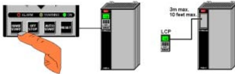
HAND START key starts the drive in Hand (local control) – speed set by + and - keys
